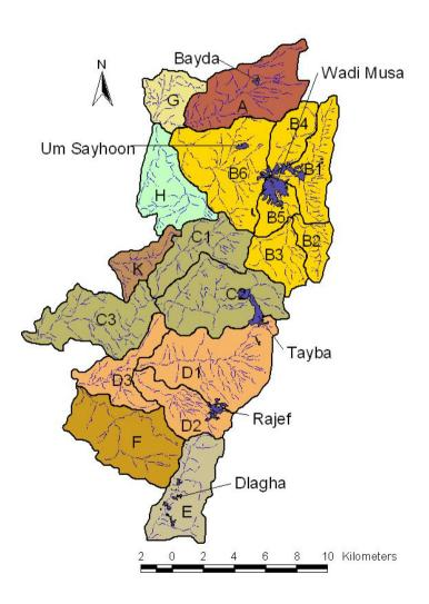
The Dlagha area is defined as according to the Watersheds E-F as shown on the graph overleaf. Catchment area E extends over about 19,820 donum. The runoff volume is based on an average annual rainfall of 150 mm and a runoff coefficient of 8% results in about 0.24 million m3. Catchment area F extends over 28,160 donum with a runoff volume of 0.34 million m3.
